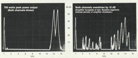
(INPUT: 14 kHz and 15 kHz - LOAD: 8 ohms, non inductive - Total spectrum sweep, 2 seconds)
