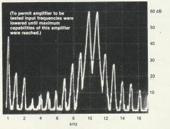
(INPUT: 10 kHz and 11 kHz - LOAD: 8 ohms, non inductive - Total spectrum sweep, 2 seconds)
