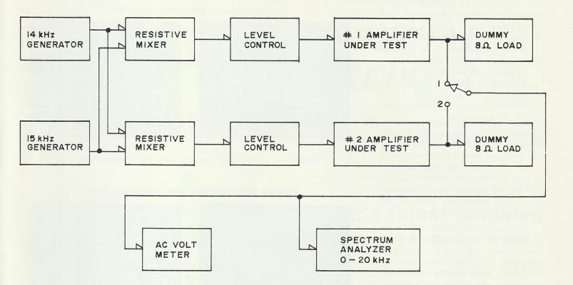
In this test set up the performance of two amplifiers can be compared. Each can have its input level adjusted independently to obtain rated power output. Then, using a switch on the adjustable level control circuit, each amplifier can be overdriven 3 dB, 6 dB or 10 dB (3 dB corresponds to asking the amplifier to produce twice its rated output, 6 dB is four times its rated output and 10 dB is ten times the rated output).
